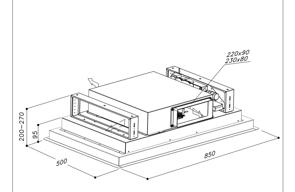
For the installation, create a false ceiling with a niche of 815mm for 465mm whose minimum height to be reached is 200mm
